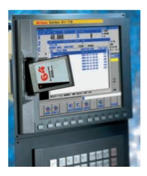
Workshop programming also has many friends, for which GE Fanuc offers special software. The highlight is the Manual Guide *i*. In version *i*, the developers have united the functionalities of the two predecessor versions, T (turning) and M (milling). With Manual Guide *i*, the user can now configure software for a turning, milling or compound machine.
